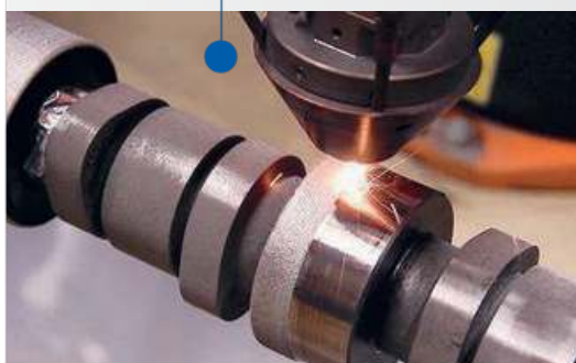
Powder cladding of flat and curved parts and of bodies of revolution
